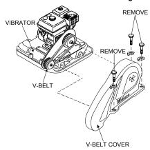
Figure 6. V-Belt Cover Removal
